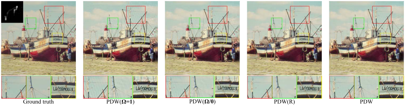
Fig. 3. Components analysis of PDW and its variants. In the sky close-ups, PDW( \Omega = \mathbf{1} ) generates significant ringing effects, while the results by PDW and PDW( \Omega/\mathbf{0} ) are visually plausible due to the partial deconvolution. Besides, the result by PDW(R) is over-smoothed due to the 30% lost entries in random partial map.
